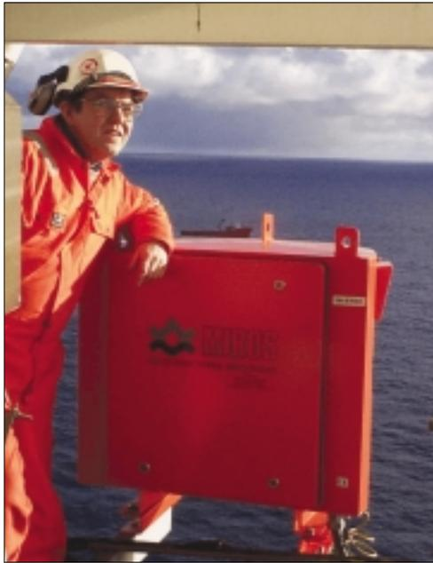
Figure 7: Miros Wave and Current Radar MkII - offshore installation
