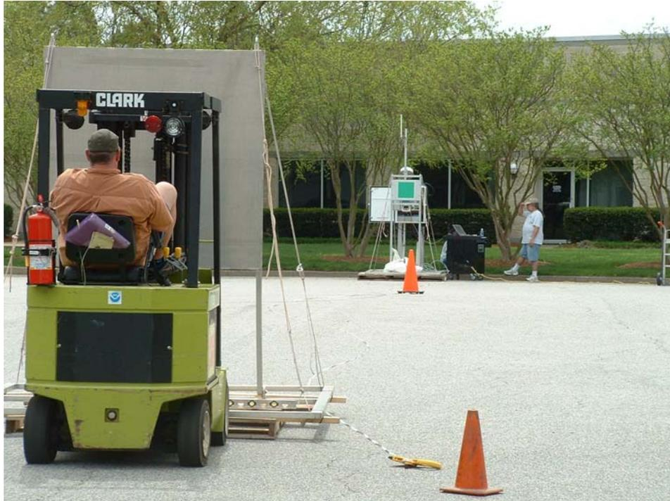
**Figure 1.** Road test in the Field Operations parking lot to compare the Miros to the universal laser sensor.
