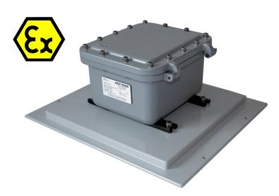
The triangular FMCW (Frequency Modulated Continuous Wave) microwave sensor accurately measures the distance to the water surface, with a sampling frequency up to 200Hz. Wave variables are calculated both from the wave point spectrum<sup>1</sup> and from time-series analysis.
